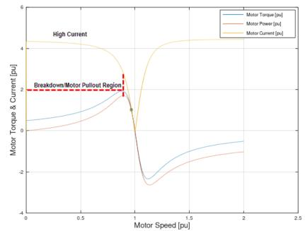
Figure 2: Normalized Power/Torque vs. Speed curve of a typical Induction Motor. If slip increases, operating speed falls into breakdown region, where motor pullout draws high current.
