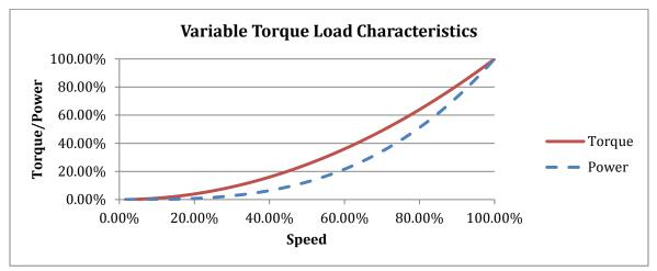
Figure 1: Power/Torque vs. Speed curve of a typical variable torque application.
