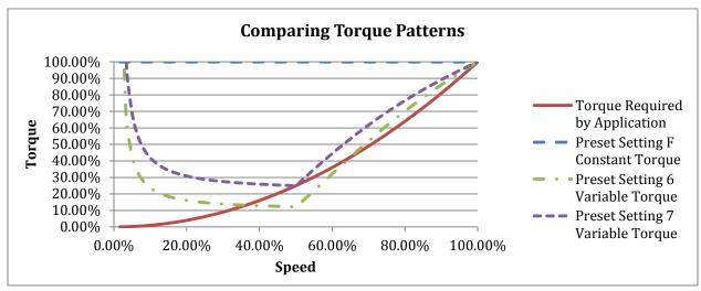
Figure 3: Comparison of preset torque patterns vs. the torque required of a variable torque application
